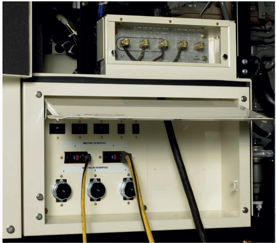
Output panels have single- and three-phase receptacles with individual circuit breakers. 120V Receptacles are energized in all voltage settings. A safety switch on the cover of the terminal connector panel opens the circuit breaker when the cover is lifted past about 30°.
